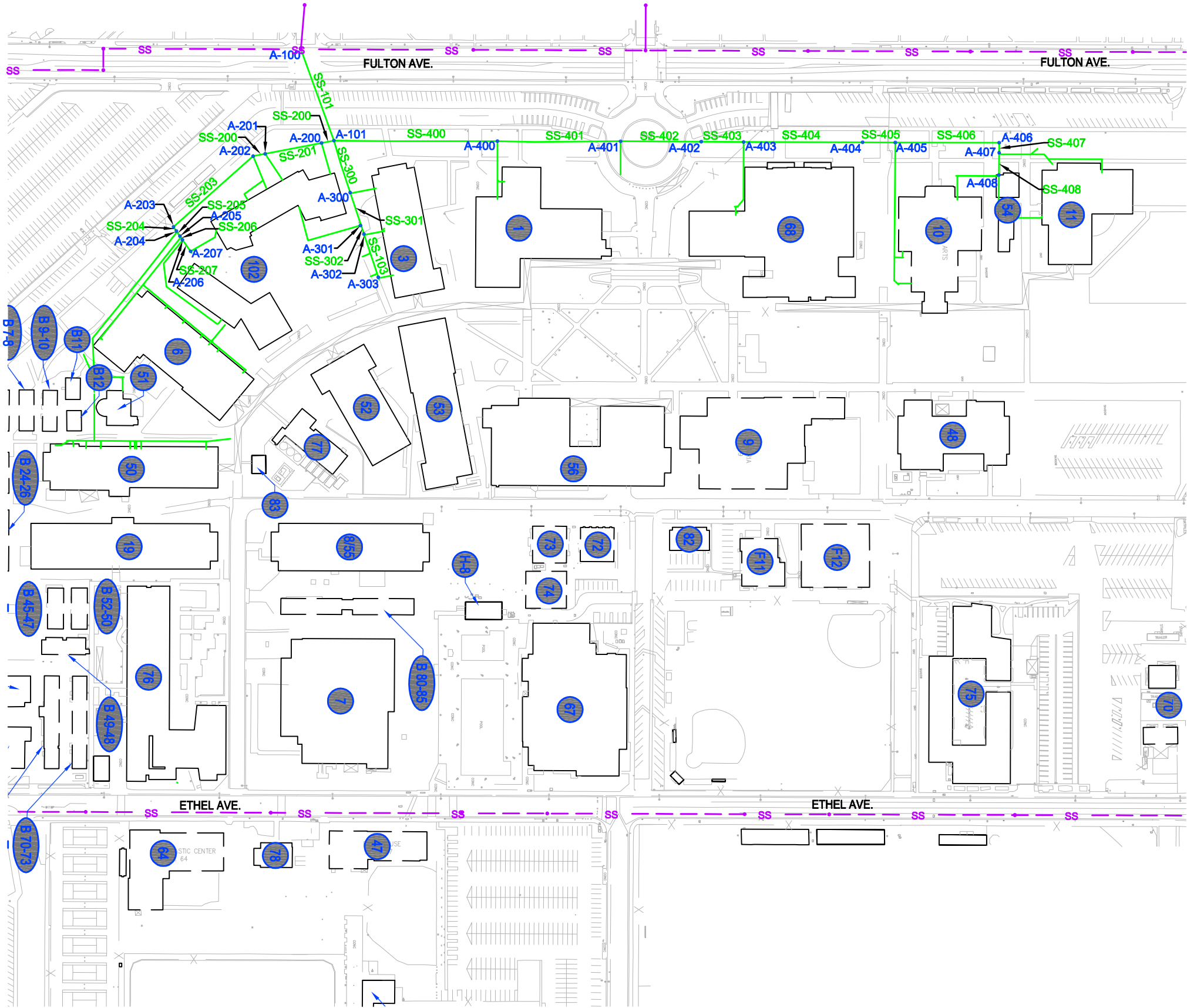
FIGURE 1d EXISTING SANITARY SEWER - PIPE AND NODE MAP AREA A
