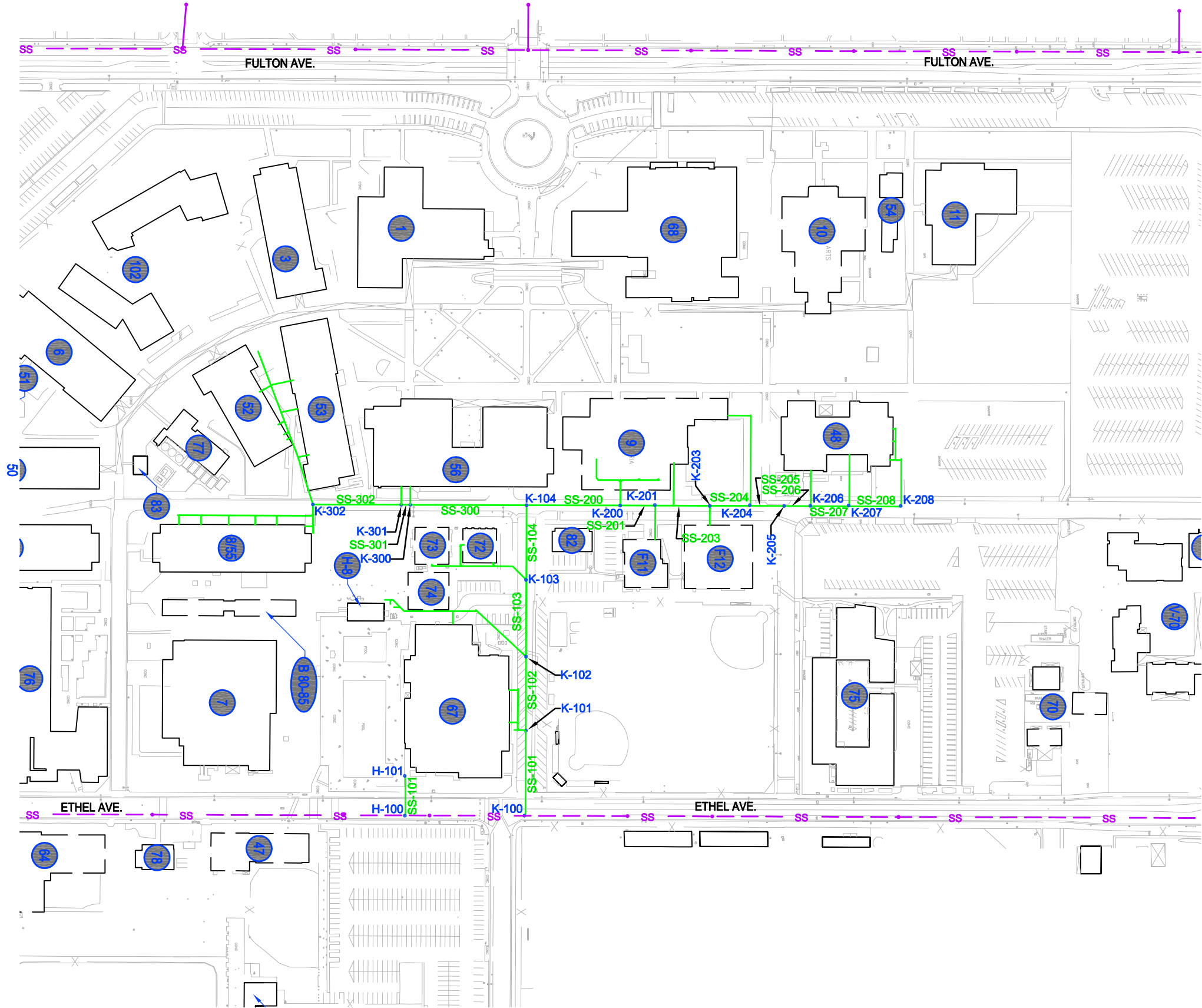
FIGURE 1j EXISTING SANITARY SEWER - PIPE AND NODE MAP AREAS H AND K
