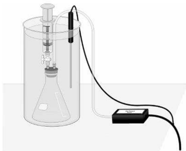
Figure 11.2. Set-up for Collecting Pressure at Changing Temperatures
